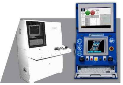
While the decades old DOS based operating systems (left) hinder friction welder production scalability, today's Windows® based welders (right) are more operationally intuitive, configurable for production scalability, and provide greater control over each weld cycle.
