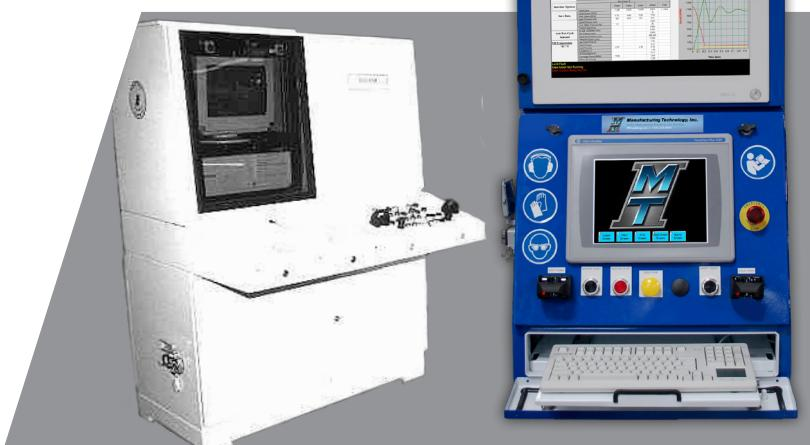
While the decades old DOS based operating systems (left) hinder friction welder production scalability, today's Windows® based welders (right) are more operationally intuitive, configurable for production scalability, and provide greater control over each weld cycle.
