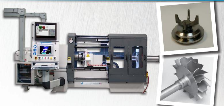
MTI is a world leader in designing and manufacturing friction welders, and offers a full line of all three main types of Rotational Friction Welding machines — Inertia, Direct Drive, and Hybrid.
