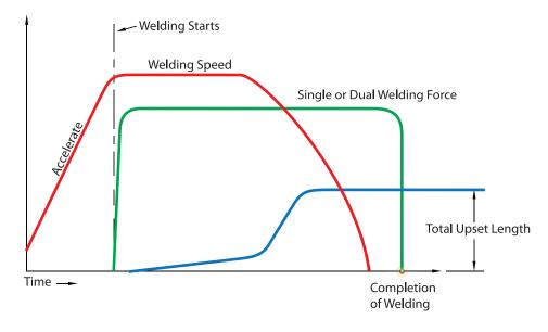
This variation combines the infinite weld energy source of the Direct Drive with the flywheel effect of Inertia. It is best applied for pre-heat on materials which need slower post-weld, cooling rates or materials which are brittle at ambient temperatures. The Hybrid process is also used for various super-alloy combinations such as large ship diesel valves or turbochargers.
