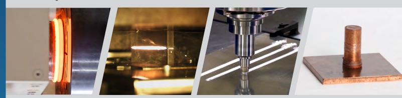
Rotary Friction Welding
