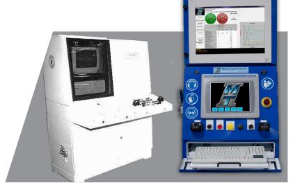
While the decades old DOS based operating systems (left) hinder friction welder production scalability, today's Windows® based welders (right) are more operationally intuitive, configurable for production scalability, and provide greater control over each weld cycle.
