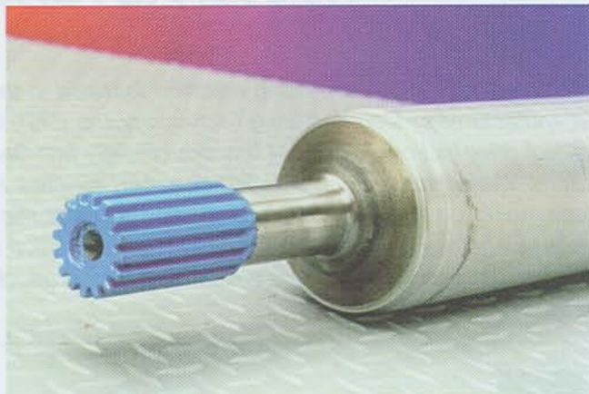
A resulting steel to aluminum bond.
